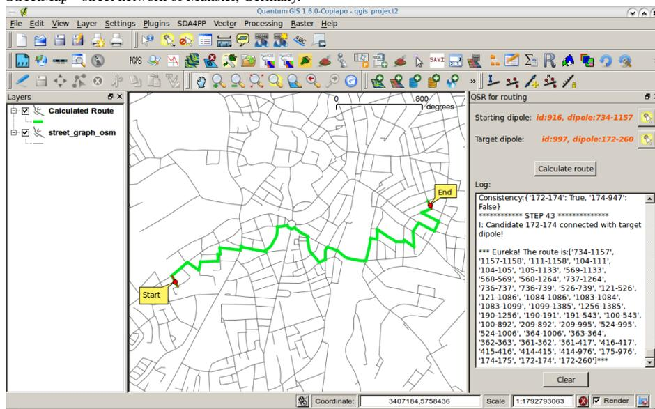
It can be noticed from figure 3 that the result is neither the shortest nor the simplest route (with regard to the number of turns) but far from being a random search. It may happen that small detours are made when picking one out of several “consistent” streets randomly. However, despite of the coarse qualitative knowledge representation provided by the Dipole calculus the navigation algorithm heads towards the target quite reliably.
